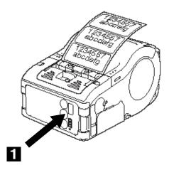
2. Press the FEED button (1) to feed a label.
